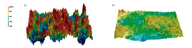
Figure 3: Surface profiles of SLS parts made of L&V TPU LUVOSINT X92A-1: a) without surface treatment, b) with VFS surface treatment. All images are stretched by factor 5 in the z-direction to better illustrate the differences in roughness.
