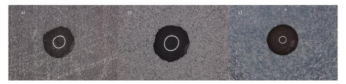
Figure 4: EOS PA 2200 parts with a water drop of  $20\mu$ L volume on differently treated surfaces. a) Water drop on colored EOS PA 2200 (r=4,5mm), b) on PSS treated and colored EOS PA 2200 (r=3,8mm), c) on VFS treated and colored EOS PA 2200 (r=2,7mm).
